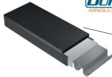
DuraSeal incorporates a unique laminating process to manufacture a versatile flexible insulating glass spacer system.
