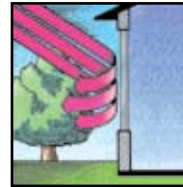
Low-E glass reflects the heat out during the hot summer months.
