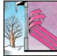
Low-E glass reflects the heat back in during the cold winter months.
